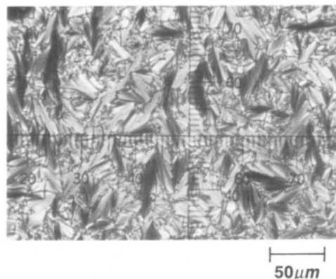
Figure 8. Optical polarization micrograph of polyOX-CN-4 annealed at 82.5 °C for 2 days.
